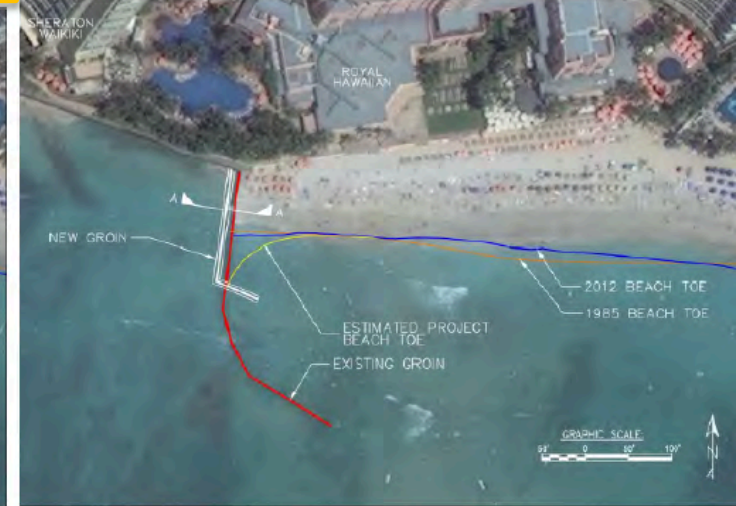
Figure 2-6 Concrete wall groin plan view
