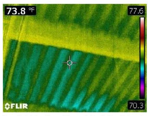
**Photo 18**: An infrared image of the area depicted in Photo 17 shows the moisture above the slab or the underlying fireproofing in this location of Storage Room 339.
