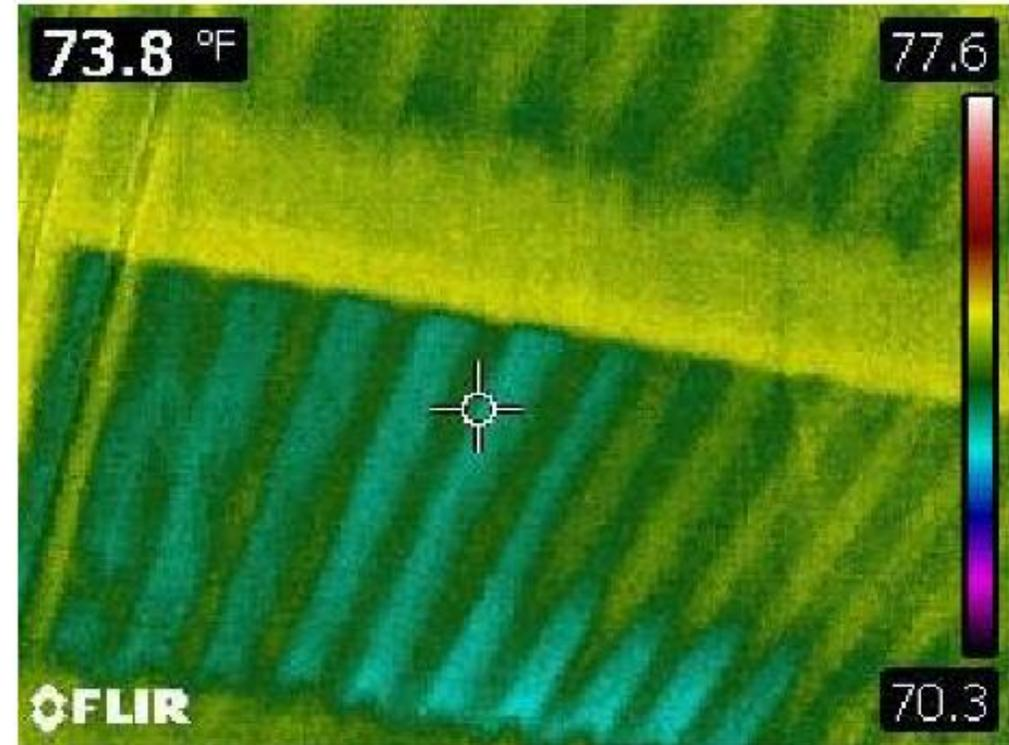
**Photo 18:** An infrared image of the area depicted in Photo 17 shows the moisture above the slab or the underlying fireproofing in this location of Storage Room 339.
